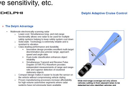
Wide mid-range coverage not only allows vehicles cutting in from adjacent lanes to be detected but also identifies vehicles and pedestrians. Long-range coverage provides accurate range and speed data with effective object discrimination.
