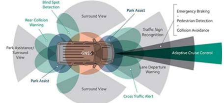
📕 Long-Range Radar 🛛 Short/Medium Range Radar 📓 LIDAR 🔄 Camera 📓 Ultrasound 📒 GNSS
